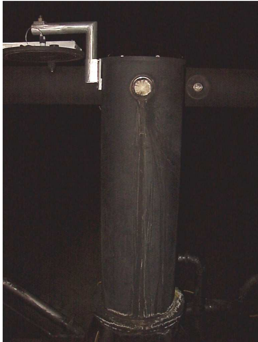
Figure 2.14: Protective enclosure, a cylindrical structure called the periscope, protects the IR camera from the hot exhaust gases and vibration from the engine. The large circle on the upper half of the periscope is a zinc selenide AR-coated window that is transmissive in the infrared. The small window to the right of the infrared window was used in previous tests for a video camera. In this photo, the top of the periscope is open to allow access to the IR camera. The shiny structure to the left of the periscope is the lid and lid support-arm.
